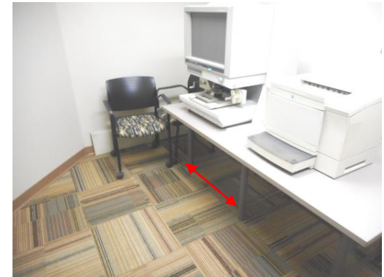
Photo 6: A microfiche machine is located in the lobby. The table holding the microfiche currently provides 25" high knee clearance that is only 28" wide (vs. 27" high minimum and 30" wide minimum).
